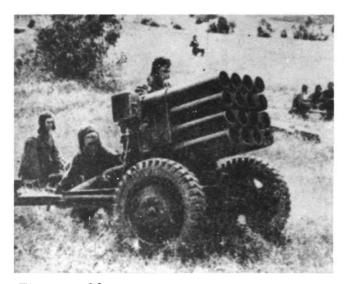
Figure 6-29. Multiple rocket launchers. The  $\bar{1}40$ -mm 16-tube BM-14 (above), towed on a two-wheel carriage, is a standard weapon in airborne divisions. Heavier rockets, such as the 240-mm 12-tube BM-24 (below), are carried on heavy trucks.
